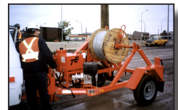
Hydraulic tensioning reel stand, skid based or trailer mounting
